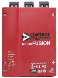
The robust design of MicroFUSION allows for continuous full-frame current operation - without derating - at up to 50° C / 6000 ft altitude. Cooling is accomplished through either natural convection, forced air, optional external panel mount, or optional liquid-cooled chill plate.
