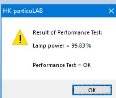
To check the performance of the laboratory device, it is possible to make a performance test with a reference cuvette.
