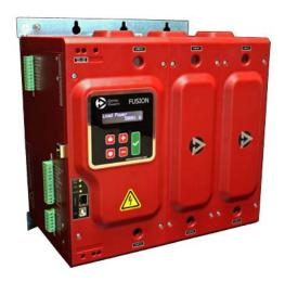
Loads can be controlled in phase-angle, zero-cross, or burst modes for operation of resistive or transformer connected loads. Output is controlled linearly with respect to command signal and can be set to the average or RMS value of the voltage or current, as well as true instantaneous power or external feedback.
