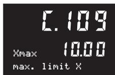
**Span end X100: (only with ratio controller)**
