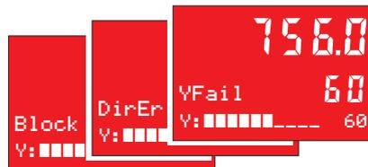
When the plant trouble was removed, the operator must inform the controller accordingly. For this, press key  or  and/or switch the controller to "automatic mode". If the actuator error continues, the controller detects it and switches off again. In any case, the controller must be switched back to automatic mode by the operator!
